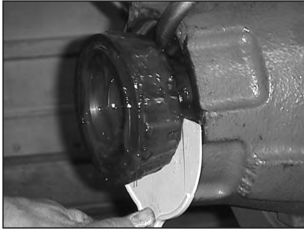
Fig. 5C: Using Template to Hold Lubricant
