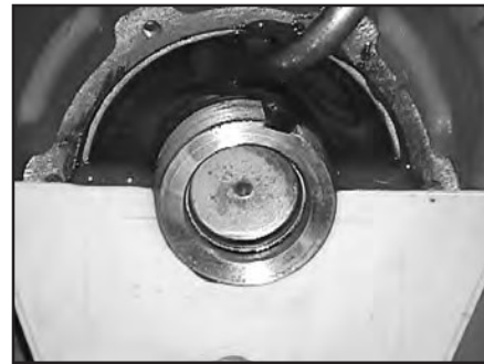
Fig. 5: Semi-Fluid Grease Top-off Procedure
